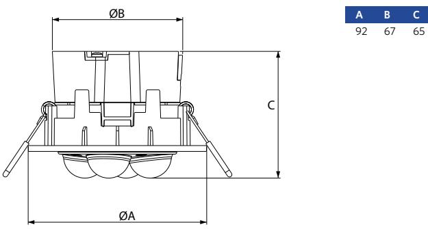
821006002000 - LEDSmart-BLE2-Rc-PIR-Sensor
